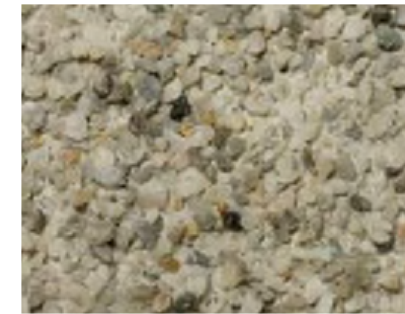
Aggregate paving - type 1 Misty gray marble
