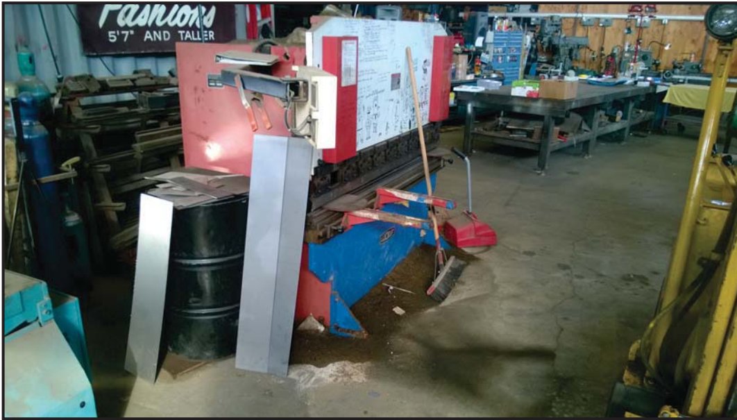
Oil staining around base of machinery.
