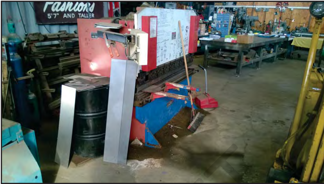
Oil staining around base of machinery.
