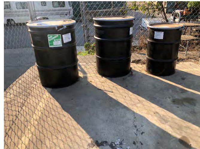
Photo 32: 55-gallon drums containing soil cuttings and purged groundwater from a 2019 Phase II investigation.
