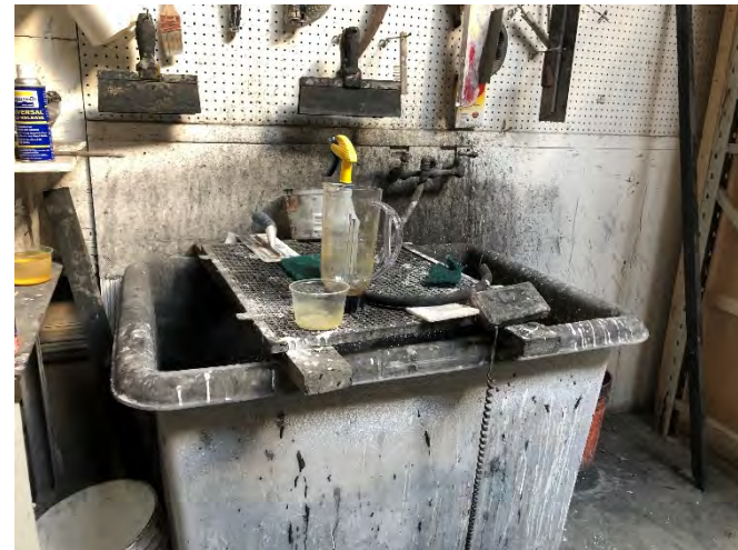
Photo 12: Paint washing basin inside Ironies. Waste is collected in 55-gallon drums for offsite disposal.
