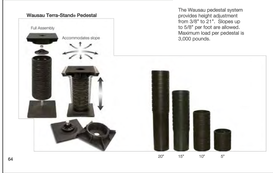
ROOF PAVER PEDESTAL SYSTEM
