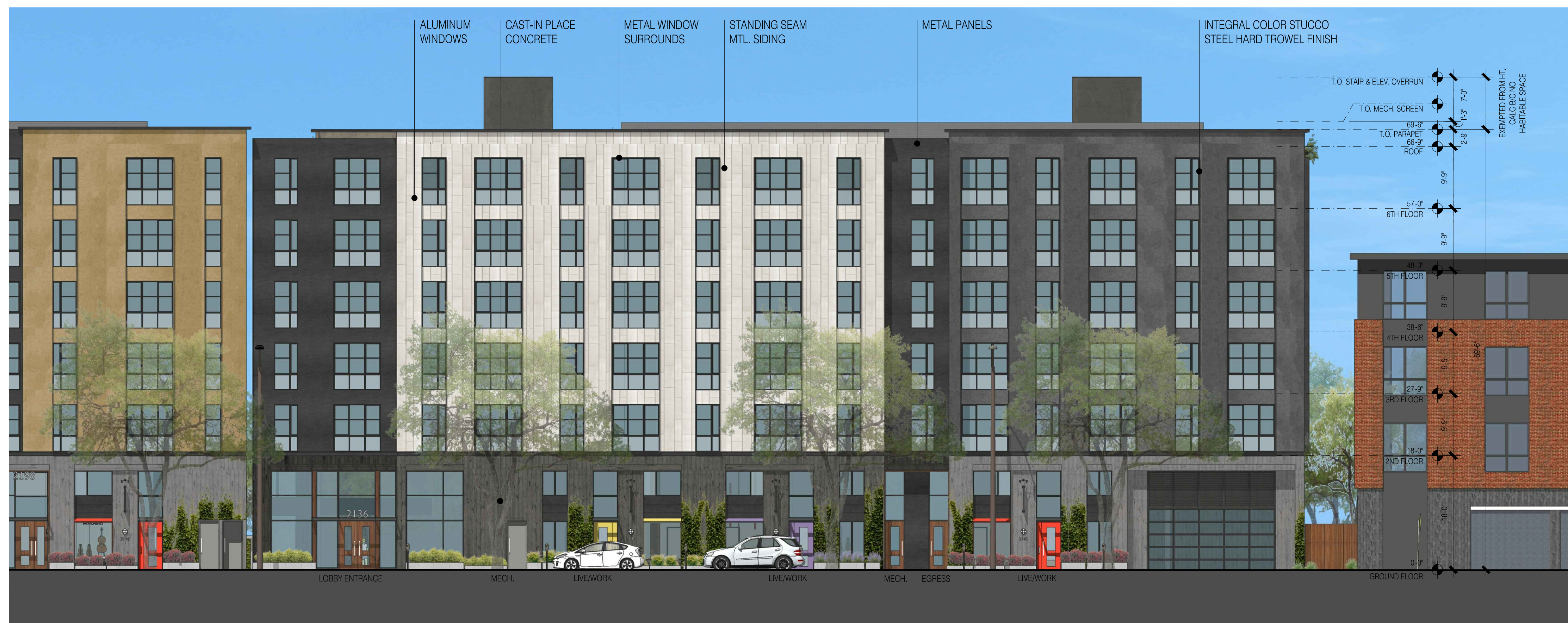
1 EAST ELEVATION 3/64" = 1'-0" @ 11X17 3/32" = 1'-0" @ 24X36
