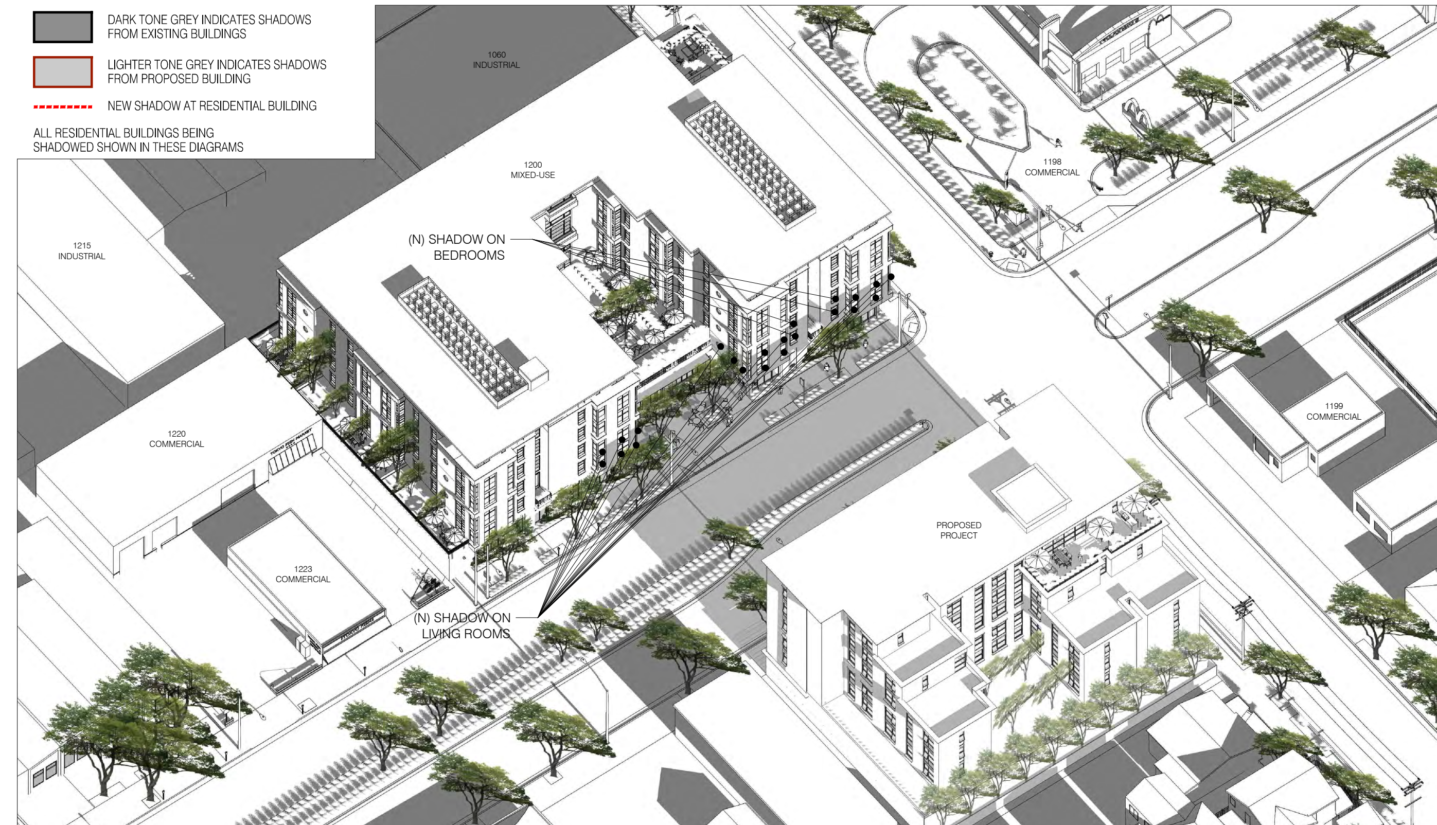
2 SHADOW STUDY AXONOMETRIC - JUNE 21: 2 HRS AFTER SUNRISE 1:100 @ 11X17 1:50 @ 24X36
