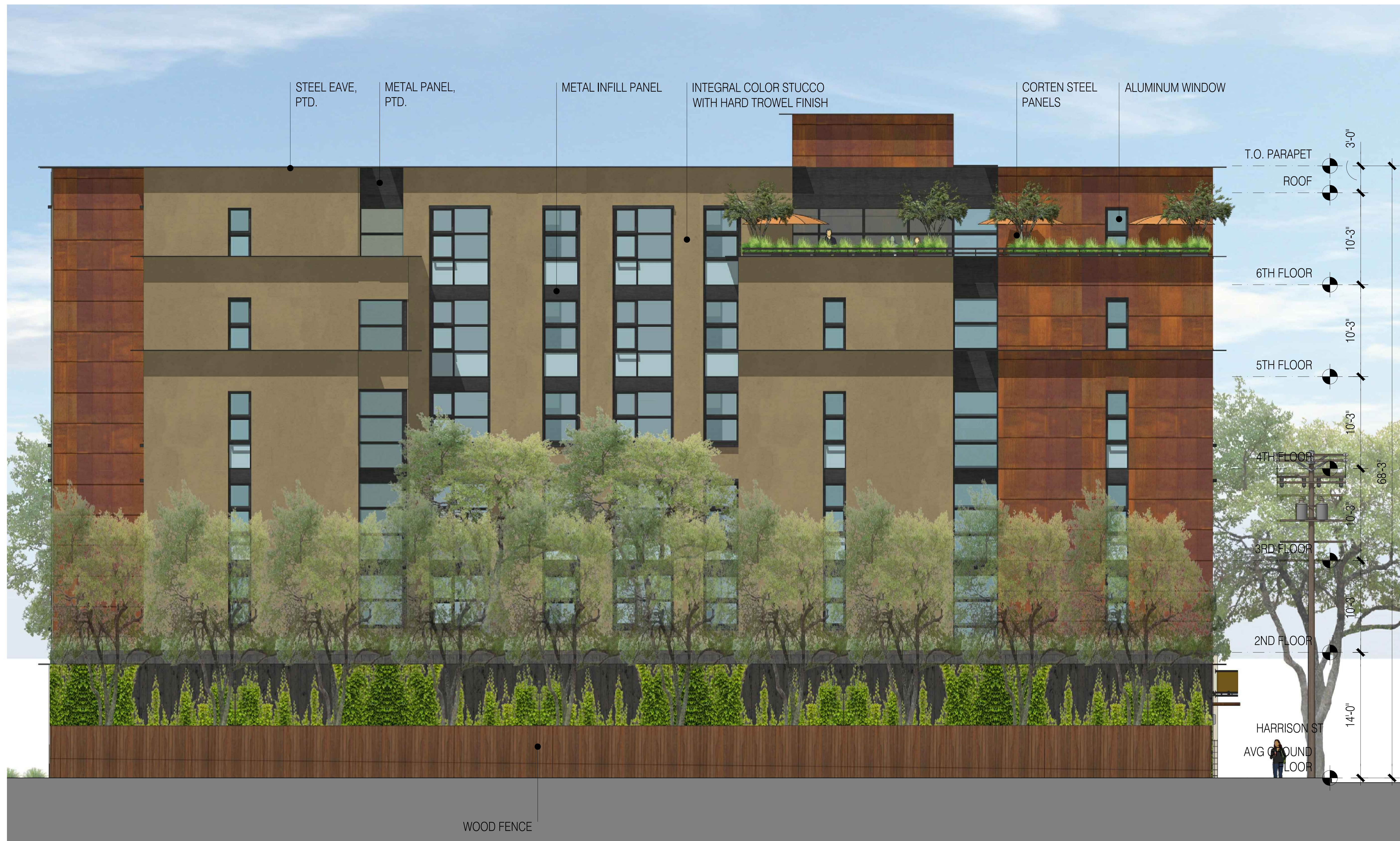
1 EAST ELEVATION 3/32" = 1'-0" @ 11X17 3/16" = 1'-0" @ 24X36 0 4 8 16
