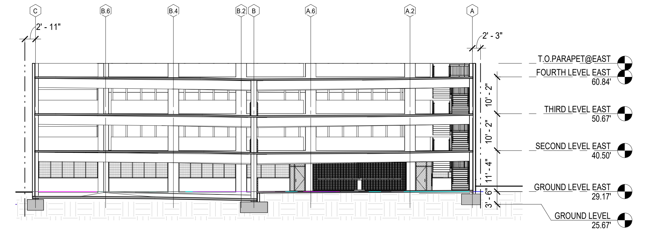
4 BUILDING SECTION 3 SCALE: 1/16" = 1'-0"
