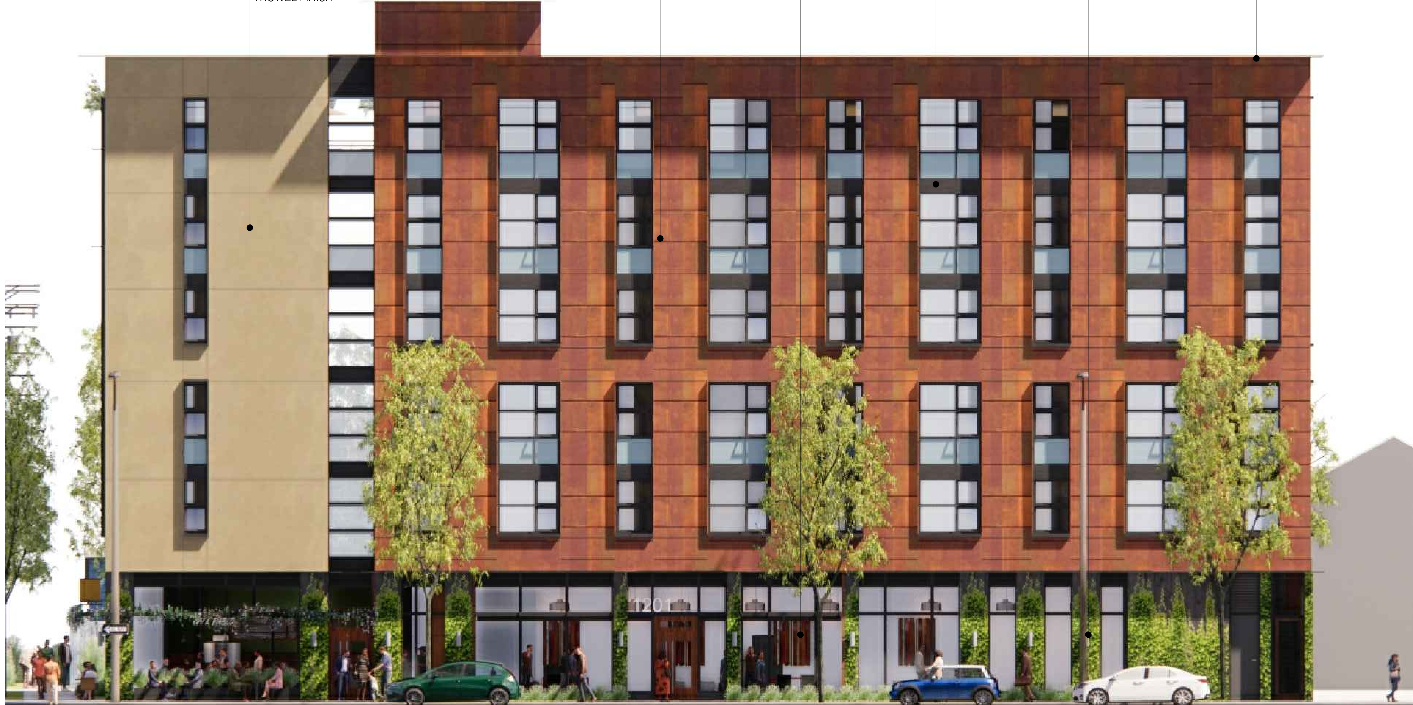
INTEGRAL COLOR STUCCO W/ SMOOTH TROWEL FINISH CORTEN METAL PANELS ALUMINUM STOREFRONT METAL INFILL PANEL CAST-IN-PLACE CONCRETE STEEL EAVE, PTD.
