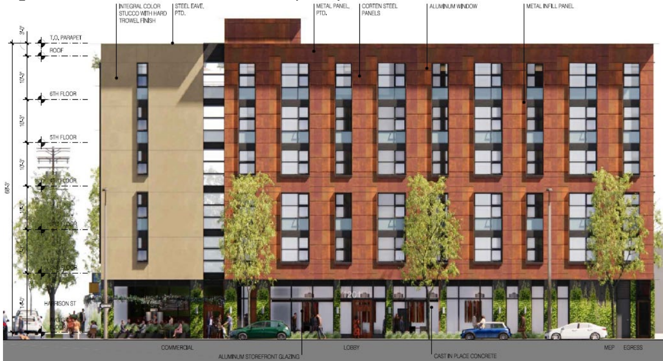
Figure 2: San Pablo Avenue Elevation (West)
