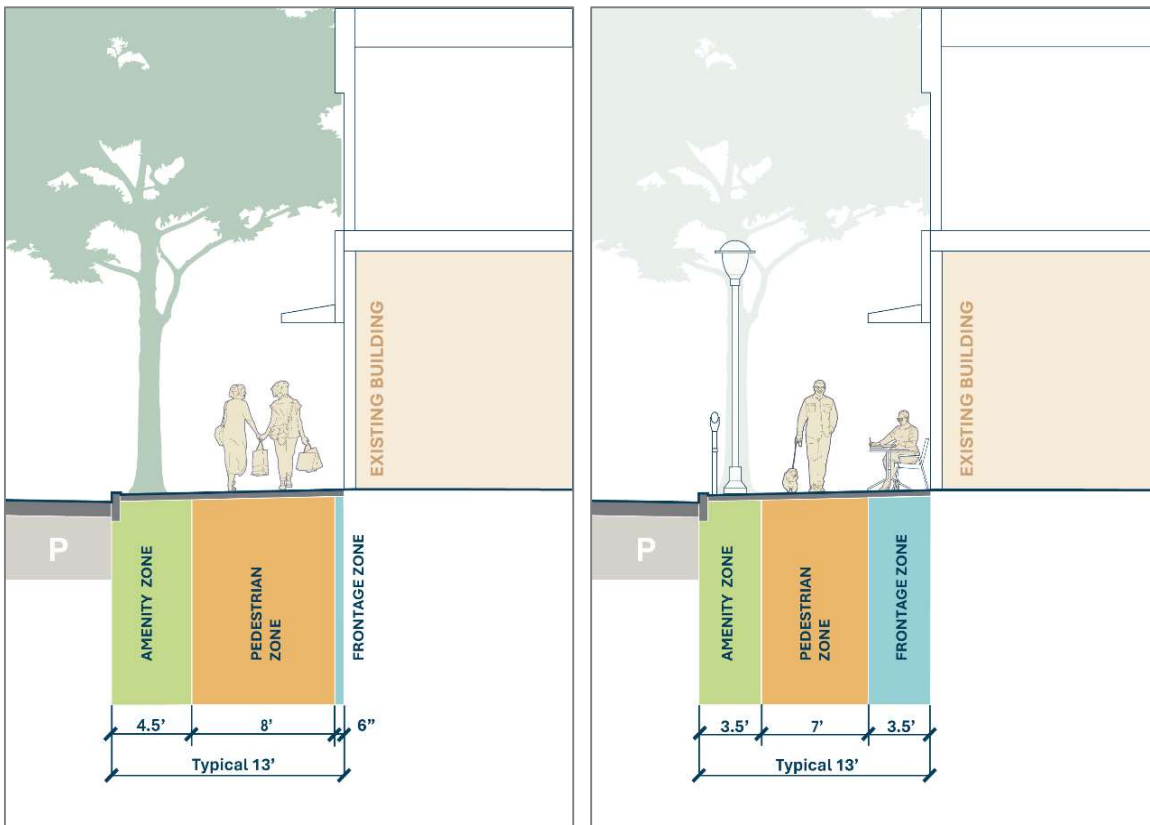
Figure 5.13 Sidewalk Zones Condition at Existing Buildings
